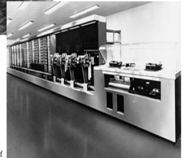
Two views of Mark I. The four devices in the centre of the pic below are the tape readers. The output typewriters are on the right.
