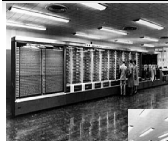
Two views of Mark I. The four devices in the centre of the pic below are the tape readers. The output typewriters are on the right.
