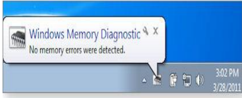
Figure 3. After reboot, the Windows Memory Diagnostic tells you, via a tooltip, what it found. In this case, the tested RAM was fine.
