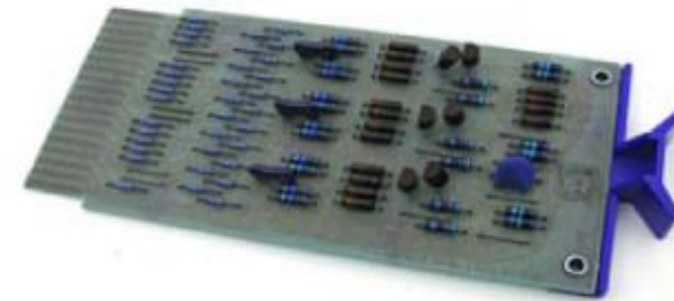
Triple flip-flop from a DEC mini-computer: six transistors, plus resistors, capacitors and diodes. The board is 125mm long, 62mm wide
