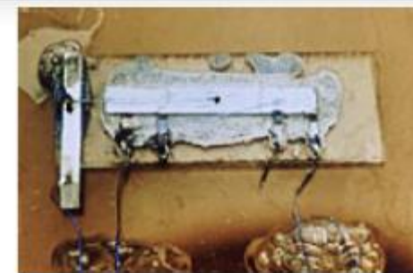
Kilby's oscillator, 1.57mm long, 1mm wide (Texas Instruments)
