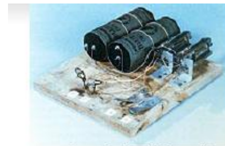
A replica of Stibitz's first adder
