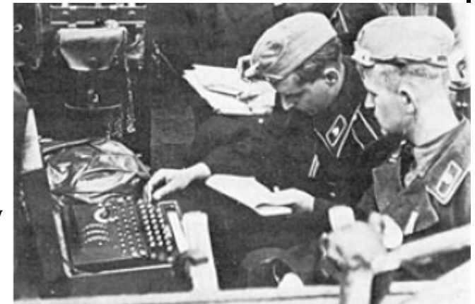
German signal staff with their Enigma machine. The three rotors can be seen. Between them and the keyboard are the letter windows with lamps beneath
