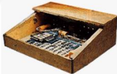
Apple I, in a home-made case. Users had to supply keyboard and monitor
